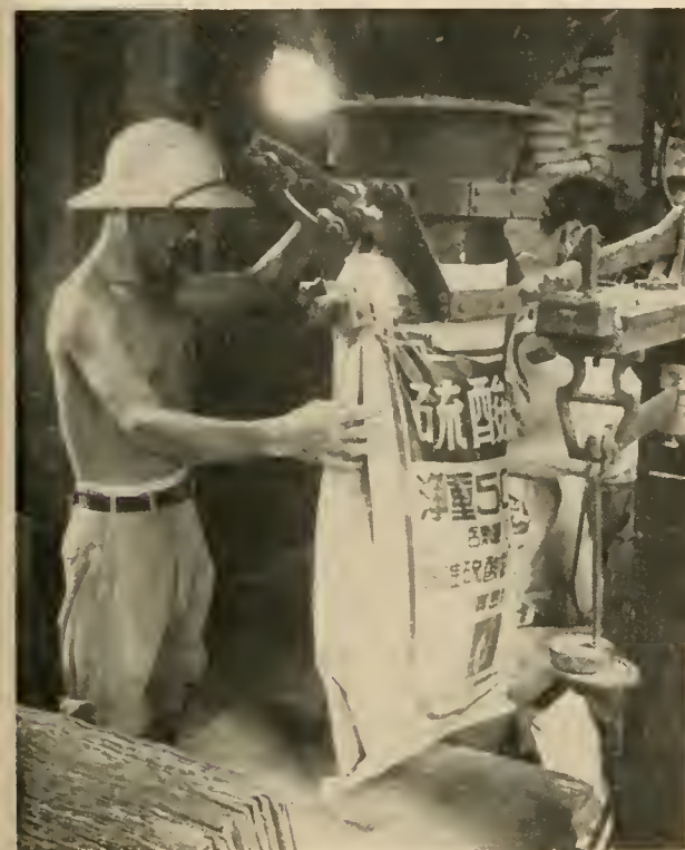
Packaging ammonium sulphate at the Kaohsiung fertilizer plant in Taiwan. This plant is being expanded to make maximum use of the island's raw materials and cut down on import requirements.
