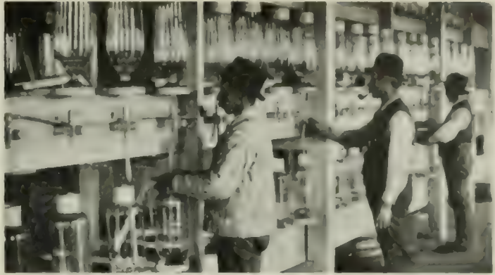
WHITEFISH EGGS KEPT IN CONSTANT MOTION IN ICE-COLD WATER
